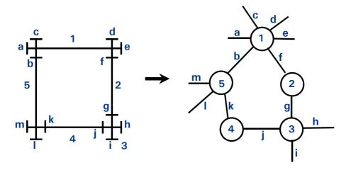
Figure 2.1. Converting a distribution map into a section diagram (Walski)
