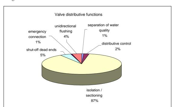
In figure 3.2 valve classification to distributive functions is shown.
